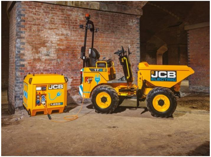
With zero emissions of  $CO_2$ , NOx and particulates, the Powerpacks are ideal for indoors and underground.
